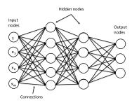
Fig. 2. Structure of a Multilayer Perceptron
