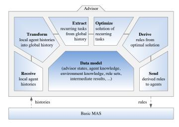
Fig. 1. EIA functional architecture
