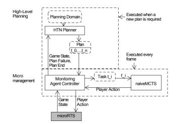
Fig. 1: Architecture of the hybrid planning and execution approach for microRTS.
