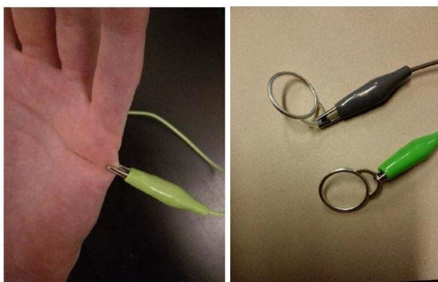
Fig. 1. Figure 1a shows Makey Makey alligator clip attached to a user's skin, very effective at conducting electricity but not too comfortable. Figure 1b shows the silver rings used to maximize conductivity and offer a comfortable experience.
